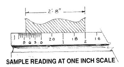
The scale for most theater drawings is 1/2" = 1'-0" though 1/4 and 3/8 inch scale are also used.
