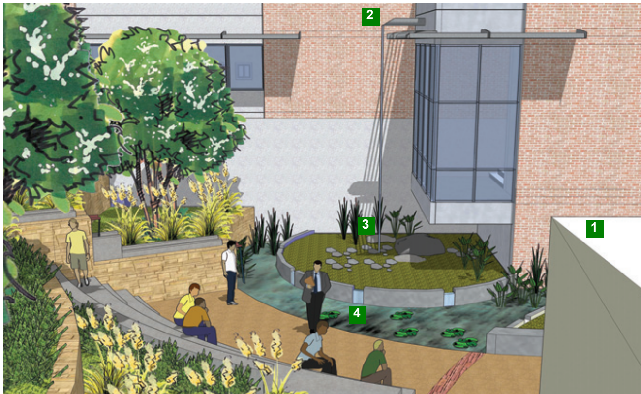
► The outdoor classroom, above, offers many scientific lessons. The white roof (1) reflects the sun and cuts energy costs. Rain water is collected from the roof (2) and funneled to plants in the outdoor rain garden (3), before feeding water into the pool (4).
